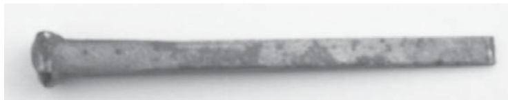
Figure 6: T-patent circa 1893 with chisel point
